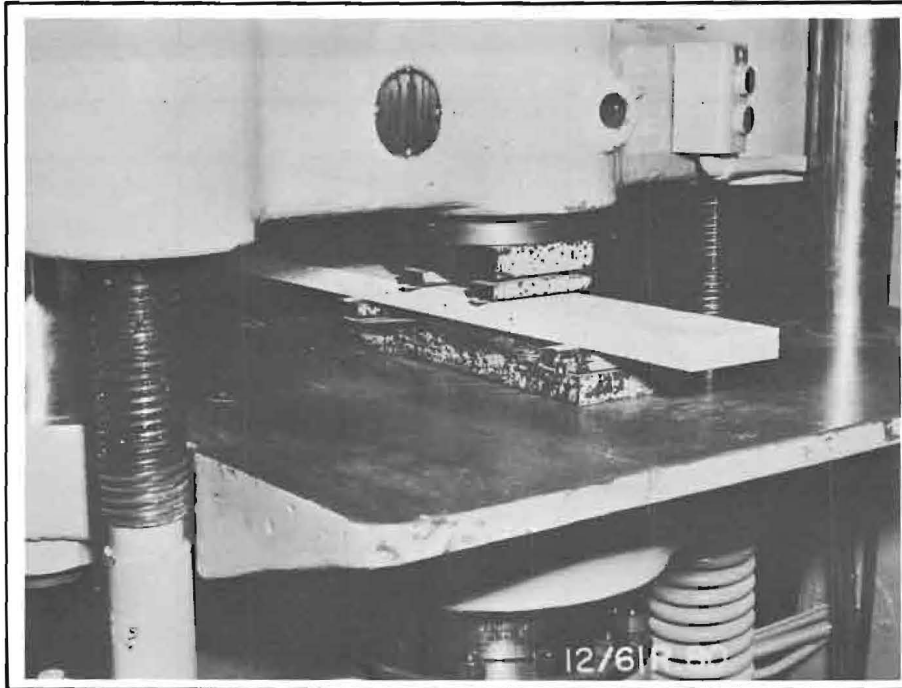
Figure 2. Set-up used for determining slab strength (flexural strength plus prestress) after completion of traffic tests. 1" x 4" x 30" beams were sawed from untrafficked areas of slabs and subjected to third-point loading.
