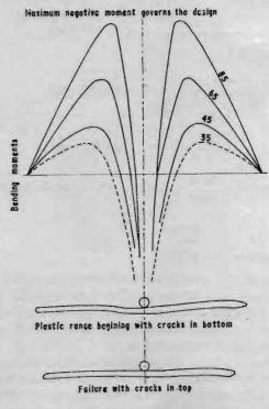
Fig 2 Bending in plastic range
