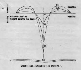
Fig | Bending in elastic range
